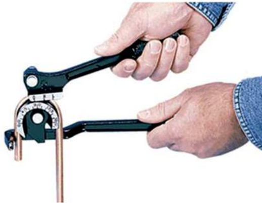
Figure 8: Copper tube and pipe bender
